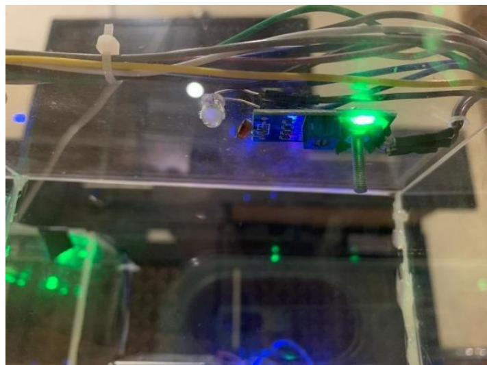
Gambar 4.16 Tampilan Sensor LDR dan LED
